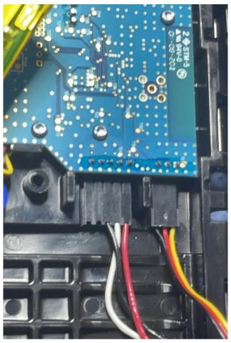
When the connectors are reattached, reassemble the board to the housing and run the self test again to see if the issue has been resolved. Take care to run the
